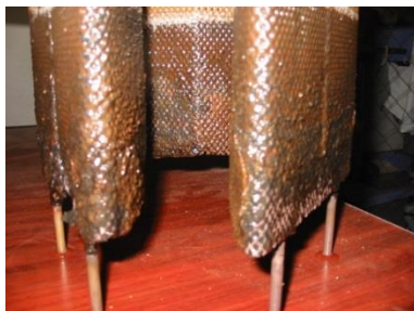
Elements soaked in pool acid solution to clean before trial commences
