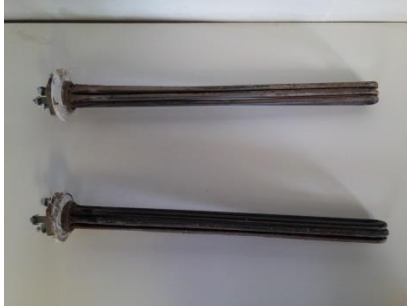
Elements after being dried in the sun and blown down with compressed air.
