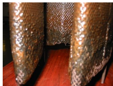
Elements soaked in pool acid solution to clean before trial commences
